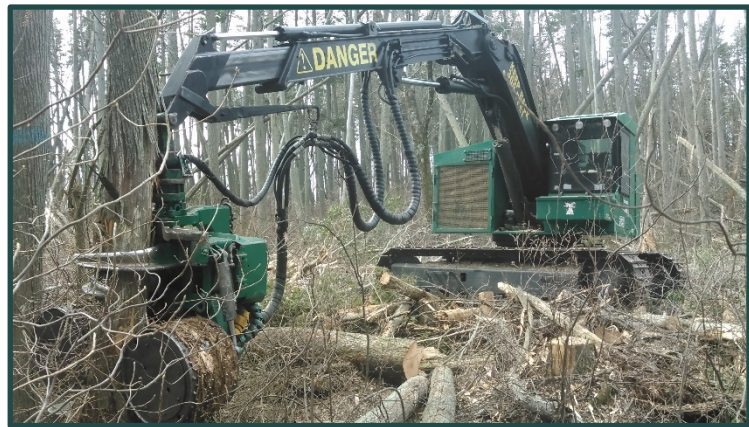
Figure 21: Tracked harvester with a cut-to-length processor head, cutting cedar in Double Trouble State Park. Similar equipment could be used for both harvesting and slashing. Source: B Isaacson, NJFS
