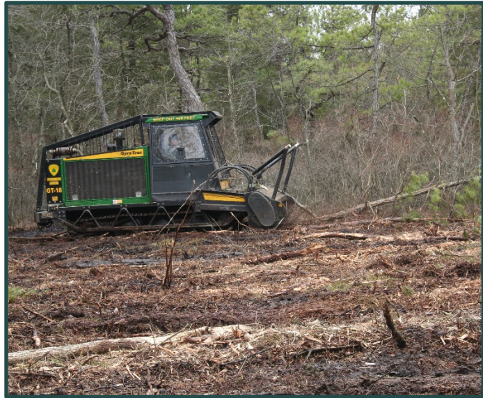
Figure 22: NJFS forestry mower clearing a site for cedar restoration. Bass River State Forest. Source: NJFS
