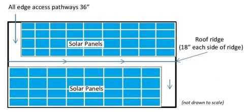
\*\* Please note, the 18" ridge setback is only allowed when the photovoltaic arrays occupy not more than 33% of the plan view total roof area when the dwelling does not have an automatic sprinkler system installed in per NFPA 13D or P2904 as per Section R324.6.2 and R324.6.2.1.
