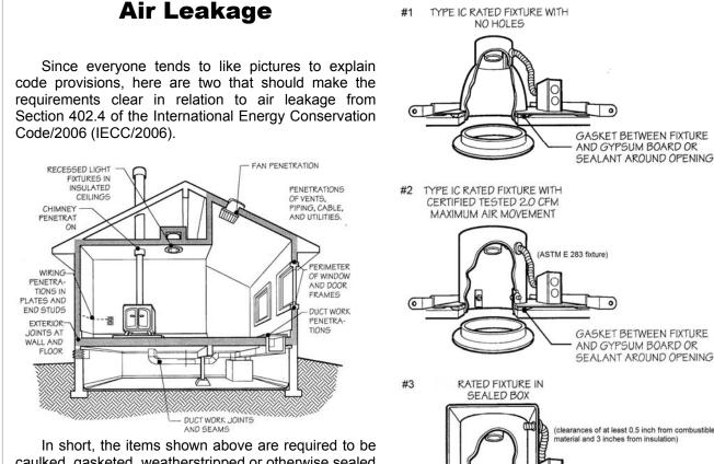
In short, the items shown above are required to be caulked, gasketed, weatherstripped or otherwise sealed with an air barrier material, suitable film or solid material to limit infiltration. The complete list of items can be found at Section 402.4.1 of the IECC/2006. Furthermore, the IECC/2006 specifically calls out recessed lighting at Section 402.4.3 to limit air leakage between conditioned and unconditioned spaces with three methods; they are as follows:
