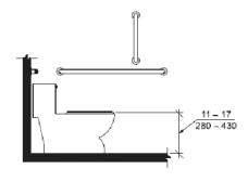
Subsection 604.10.5, Grab Bars, states that grab bars for water closets shall comply with Section 604.5.
