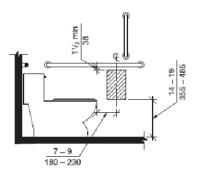
Subsection 604.10.8, Toilet Compartments, states that toilet compartments shall comply with Sections 604.8 and 604.9, as applicable.
